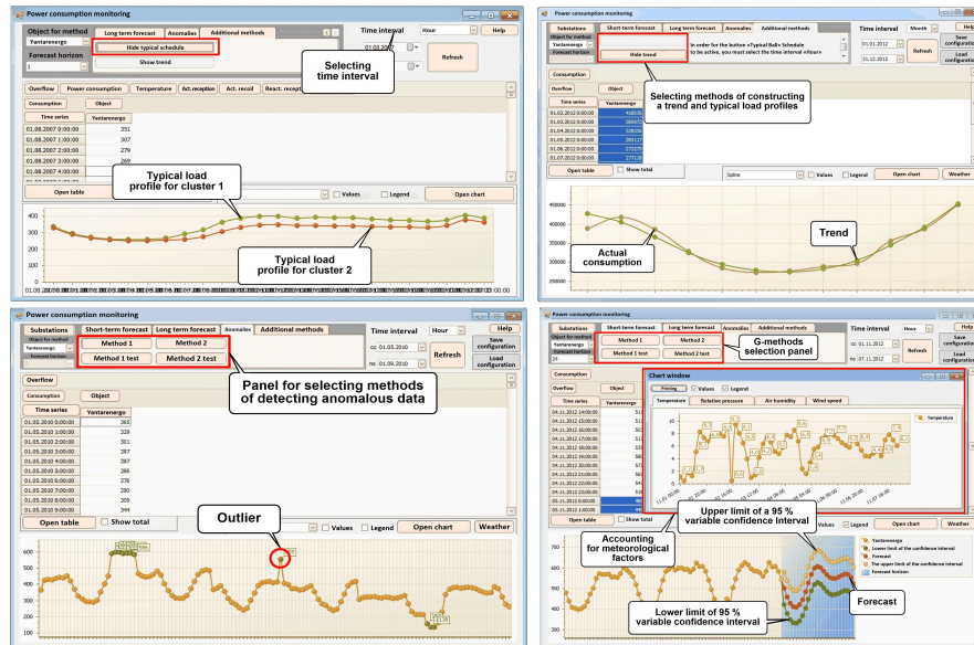
Fig. 8. Fragments of elements of the software and hardware complex monitoring power consumption of regional transport network complex of AO “Yantarenergo” [6].
