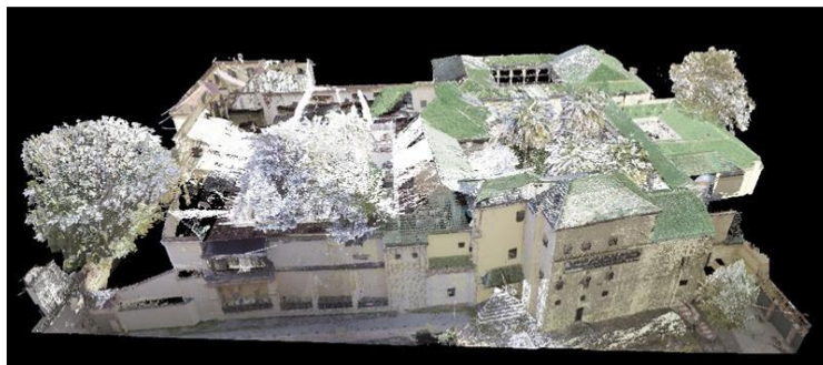
Figure 2: 3D Point Cloud model of the Ahmed Bey's Palace viewing in Cyclone software [7].
