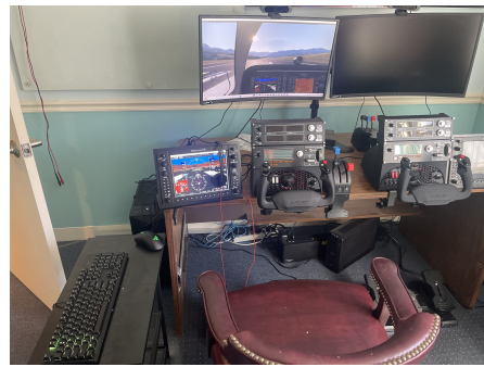
Figure 1: The flight room is where participants are tested under each scenario in MSFS. Each primary control surface has its own dedicated external device that mimics the tactile feel of real-world flight controls.
