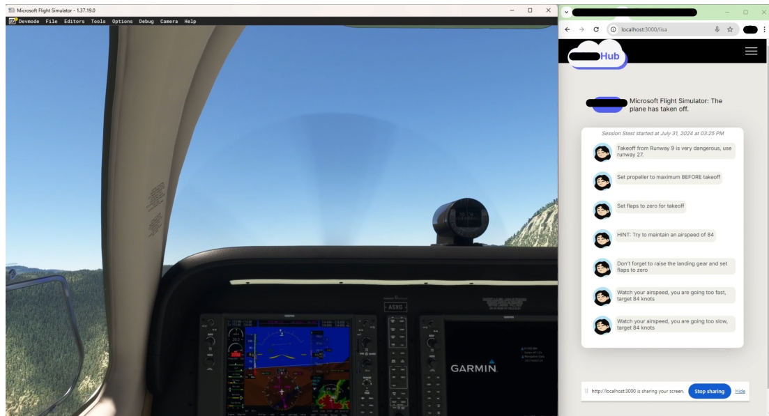
Figure 2: LISA outputs are presented on the right of the screen while the participant flies in the simulator. First LISA warns of the dangers of taking off from runway 9, then reminds the pilot to set the propeller and flaps before takeoff. Once off the ground, LISA states an ideal speed for climb, reminds the pilot to raise the landing gear, then provides time-critical alerts related to airspeed.
