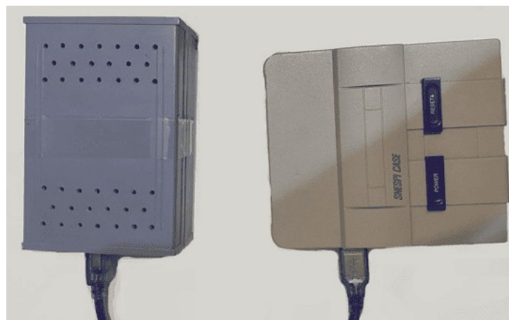
Figure 4: Indoor Air Quality Sensor in cases.
