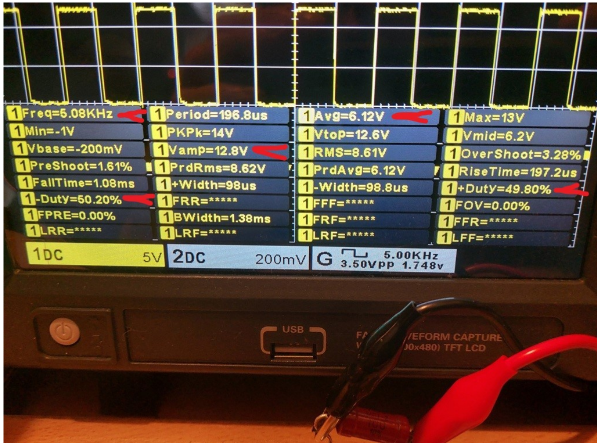
Figure 3: A photo of the screen of the DSO2000 oscilloscope from Hantek Technologies Co. Ltd. during the measurement of the average voltage Avg = 6.12\text{ V} of a sequence of rectangular pulses.
