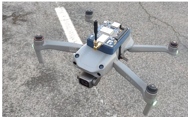
Figure 3: Test UAV equipped with the custom UWB/XBee board.
