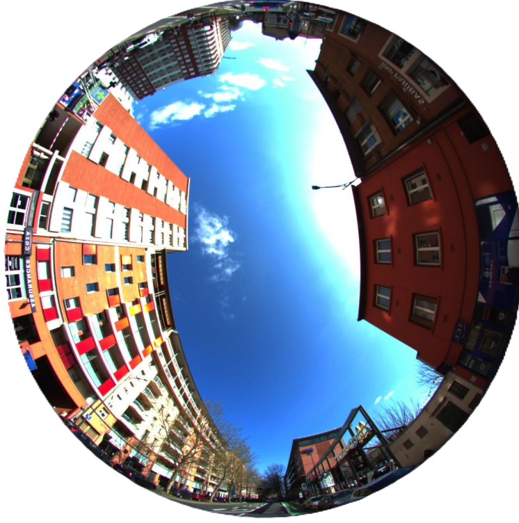
Figure 4: Image taken by the sky-facing fisheye camera used for NLOS and context classification
