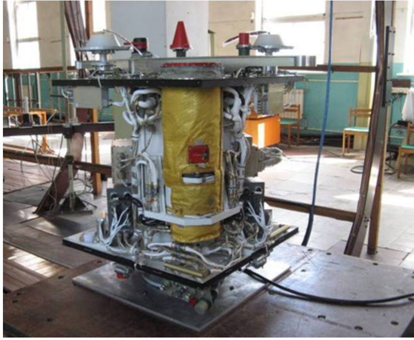
Figure 1: The spacecraft "SICH-2-1" on the measuring stand.
