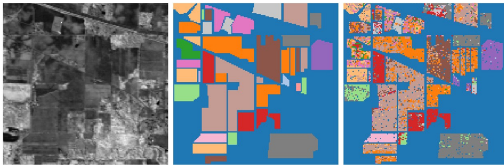
Figure 7: Prediction maps for Indian Pines dataset (5% training ratio). Figure shows spectral band, ground truth, and classification result
