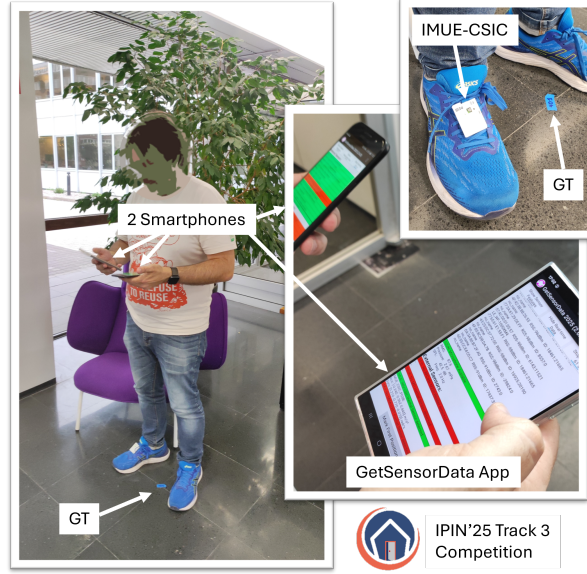
Figure 1: Illustration of the data collection setup during the IPIN'25 Competition (Track 3), showing the two smartphones running the GetSensorData App (release June 2025), the GT marks placed on the floor, and the foot-mounted IMU (model IMUE-CSIC).
