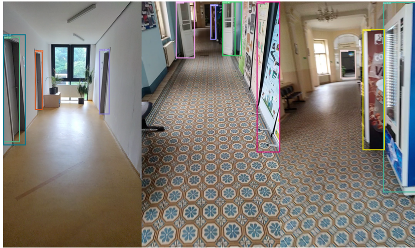
Figure 4: Door detection examples: the first image shows duplicate detections of a single door; the second illustrates various objects incorrectly identified as doors; the third shows vending machines mistakenly detected as doors. Only first image is from Scenario 1.
